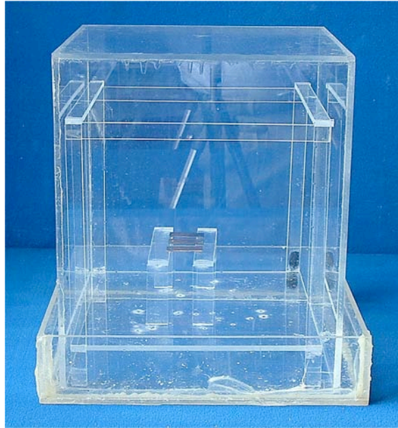
Figure 1 Thioacetamide Test Chamber
