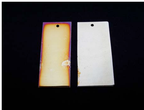
Figure 2 After 10 hours exposure in Thioacetamide chamber
